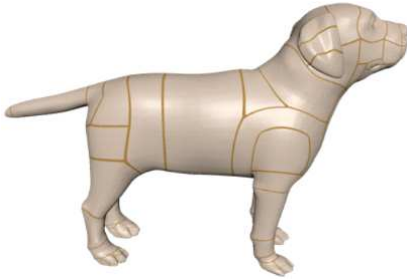
Fig. 2. ODE surface and boundary and control curves [14].
