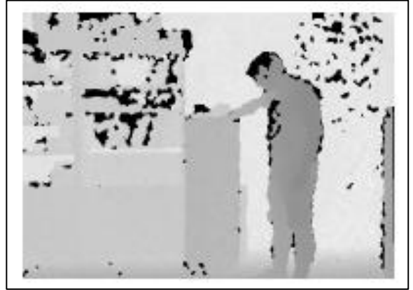
Fig 2. The pixels of the depth map in hole region that are represented by the black pixels (“non-available” Kinect tags.) [6]
